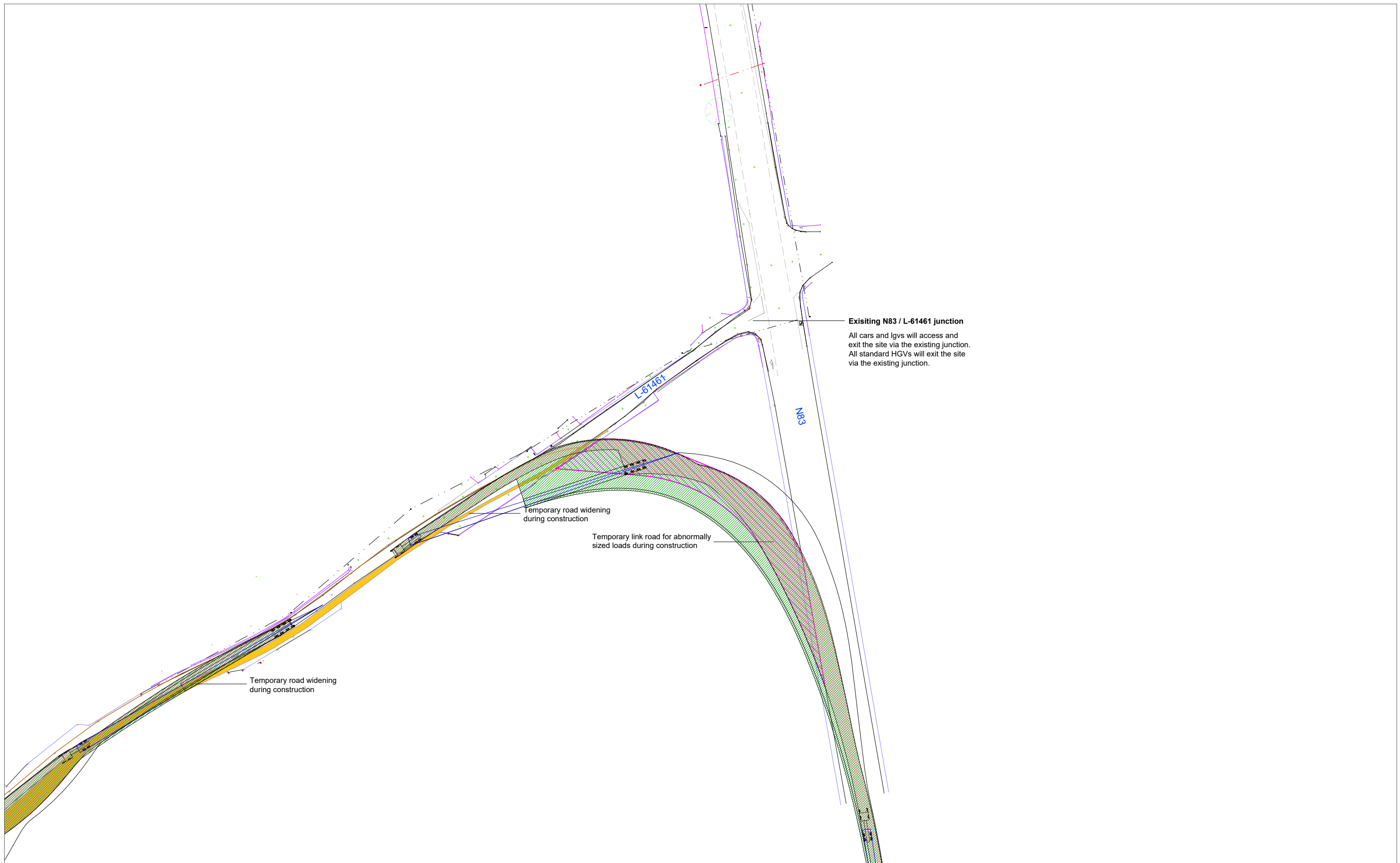
Figure 15-13 Location 4 - N83 / L-61461, proposed temporary access for abnormally sized loads and standard HGVs during construction phase - blade extended artic
