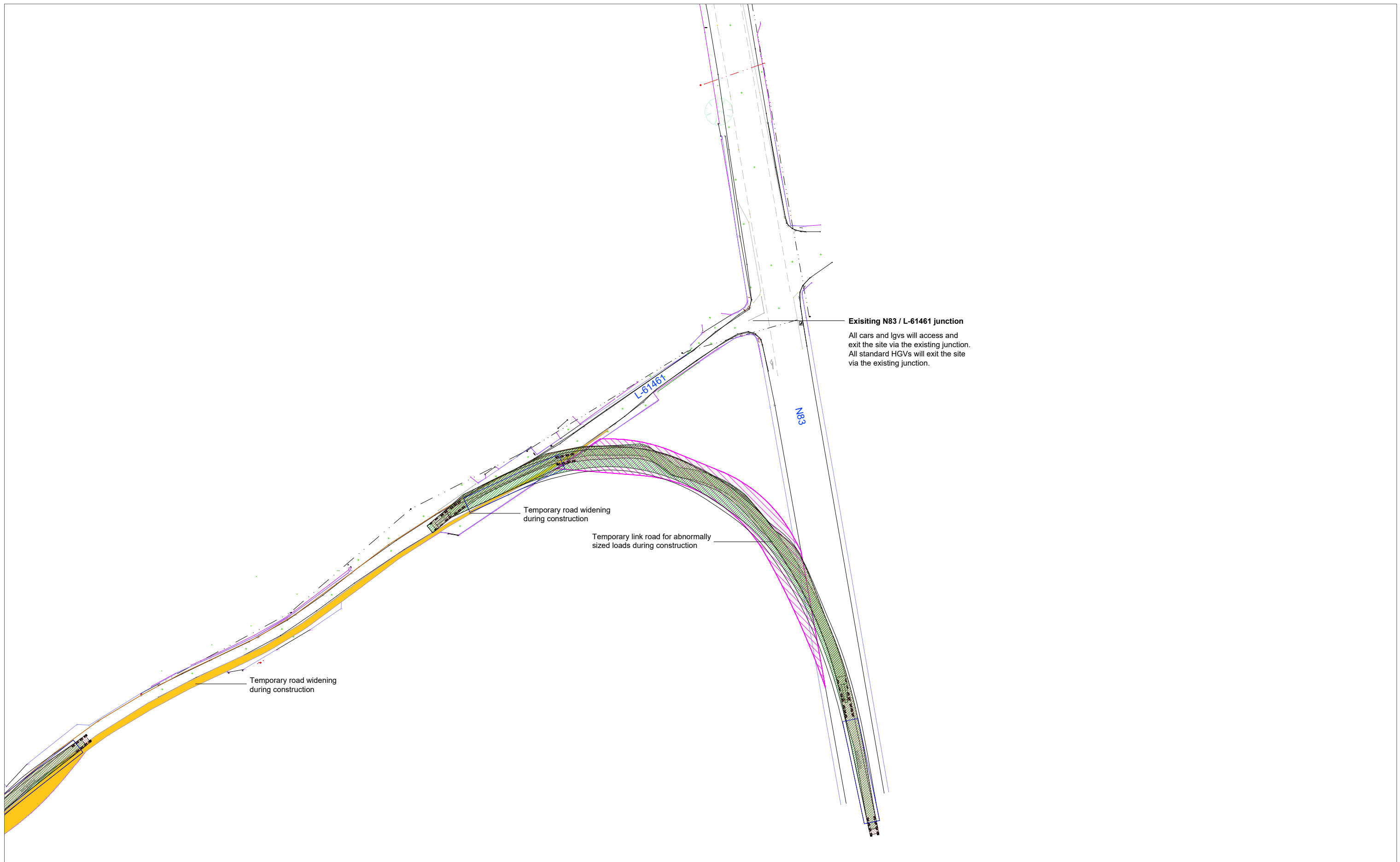
Figure 15-14 Location 4 - N83 / L-61461, proposed temporary access for abnormally sized loads and standard HGVs during construction phase - tower extended artic
