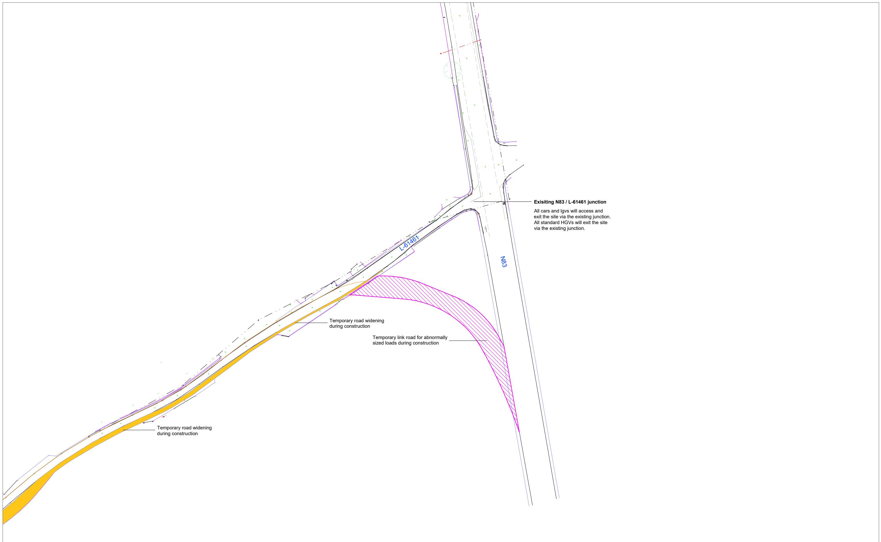
Figure 15-12 Location 4 - N83 / L-61461, proposed temporary access for abnormally sized loads and standard HGVs during construction phase
